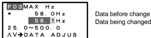
Figure 7.10 Screen Samples for Changing Function Code Data
