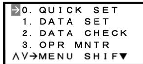
To display this menu screen, press **PRG** key in Running mode to switch to Programming mode.
