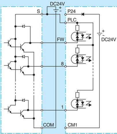
Hitachi EH-150 series PLC Output Module EH-YT16 SJ700
