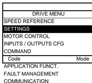
Automatically switches to the [DRIVE MENU] menu after 3 seconds. Select the menu and press ENT.
