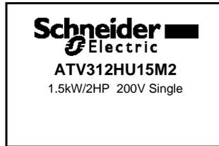
Display after the drive has been powered up for the first time.
