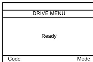
The word "Ready" appears on the graphic display terminal if you press the ESC key when in the [DRIVE MENU].
