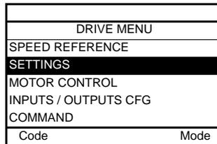
Automatically switches to the [DRIVE MENU] menu after 3 seconds. Select the menu and press ENT.
